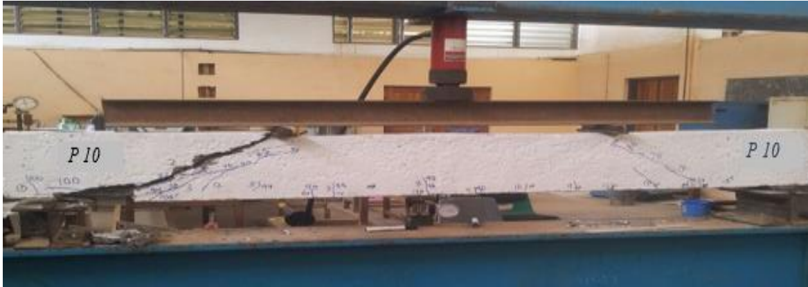
Figure 2. Test set up, instrumentation and failure mode.
